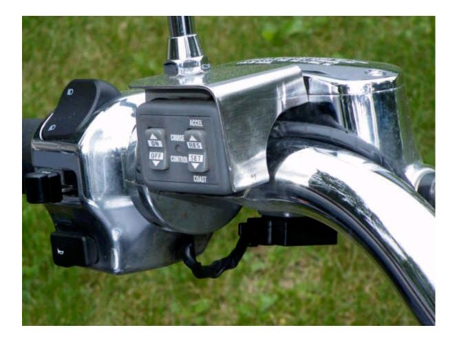
18. After you are satisfied with your bracket, you might need to lengthen your wires from the control unit. Temporarily mount the control switch to the bracket but don't peel the backing off the mounting tape. Use a rubber band to hold the control in place.
