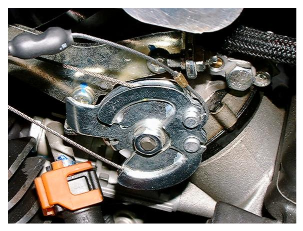
11. The Rostra only comes with one loop cable, but this picture will give you an idea of what it looks like. Remove the motor mount brace on the left side to give you access to the bellcrank on the throttle body.
